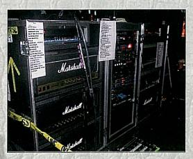
DIRTY SOUND One 100-watt Marshall JCM Slash 2555 Signature Model head run in parallel with one 100-watt Marshall Vintage Modern head-each driving a Marshall 4x12 straight cabinet. For extra distortion, volume, and dimension during solos, Slash's tech typically kicks in the Overdrive section of an MXR/Custom Audio Electronics Boost/Overdrive pedal, and some delay from a Yamaha D1500 rack unit placed in the Vintage Modern's effects loop. Occasionally, the latter amp's preamp section gets an
